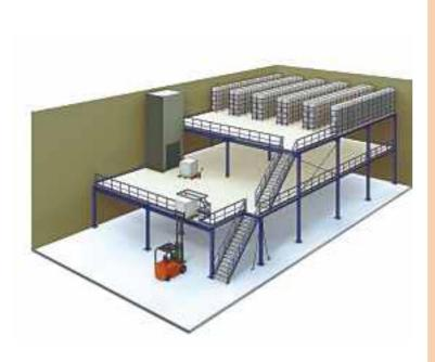
The Giraffe Mezzanine racks can increase the storage capacity of any place to a great extent. Giraffe Mezzanine Floors create extra floor space by using heavy duty structural steel section decked in, steel plates or open mesh to create a second storey. Whether your requirement is simple or complex, when you buy your storage solution from GIRAFFE you will benefit from our vast knowledge of maximising warehouse and office usability and efficiency.
