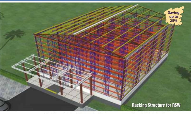
In lieu of Storage Racks installed in Conventional Warehouses, we propose an Economical Solution by making a Rack Supported Warehouse (RSW), where apart from storage, Racks also undertake all the evenly distributed Loads of Superstructure and sheets as an Integrated Structure. Having Direct savings upto 25% in Cost of PEB Structure and also Civil Construction by Eliminating Heavy Foundation Footings, we have successfully installed many RSWs in India and abroad, in last 8 years.
